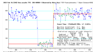
図 8: We analyzed the video shown in Figure 6, and then fit the diffraction simulation model to the light curve of the star occulted by the asteroid to obtain the most likely value of the event time. As a result, we found that 17^{\text{h}}43^{\text{m}}22.785 \pm 0.021\text{s} was the most likely value of the event time. This means that the event occurred 0.081s before the timestamp of 17^{\text{h}}43^{\text{m}}22.866\text{s} , which is the timestamp of the frame in which the faint star image was seen.
